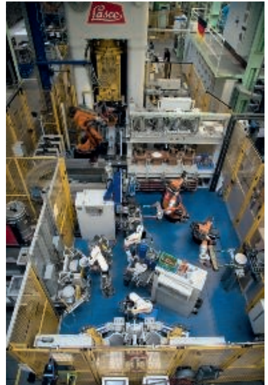
WHERE RAW FORCES ARE USED SENSIBLY The bases of all WMF pots are pressed with a force of up to 1300 tonnes at temperatures of over 500 °C. This is what makes them especially robust.
