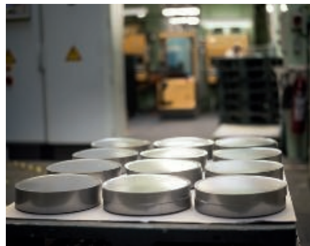
RAW MATERIALS LINED UP All WMF pots have a TransTherm® universal base. Its core consists of solid aluminium for optimum heat conduction and storage.
